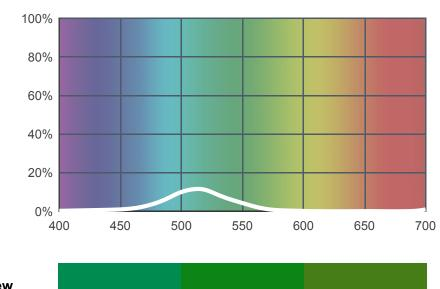
**Light transmitted (Y%)** for each colour wavelength (nm)
