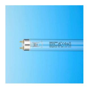
Germicidal lamps efficiently emit a large amount of ultraviolet rays 253.7nm (nanometers) which have excellent germicidal effect. These lamps have structures and electrical characteristics similar to those of general fluorescent lamps used for illumination but use ultraviolet ray glass which efficiently transmits ultraviolet rays at 253.7nm.
