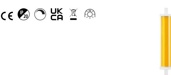
ToLEDo R7s is a retrofit replacement for traditional halogen double-ended linear R7s lamps The slim design and glass construction give the same look and feel of traditional halogen R7s lamp Omni-directional light distribution High lumen efficacy Lumen output: 850lm 85% energy saving Length: 118mm Non-Dimmable 15,000 hours average rated life Ideal for domestic and commercial applications
